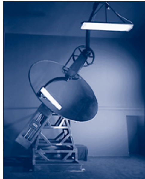
CEAG products are constantly being advanced and tested in the company's own lighting laboratory
